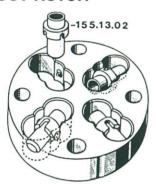
The Swing-out ROTOR type 154.120.U is available with 4 type 155.13.02 holders for type "H" inserts.
